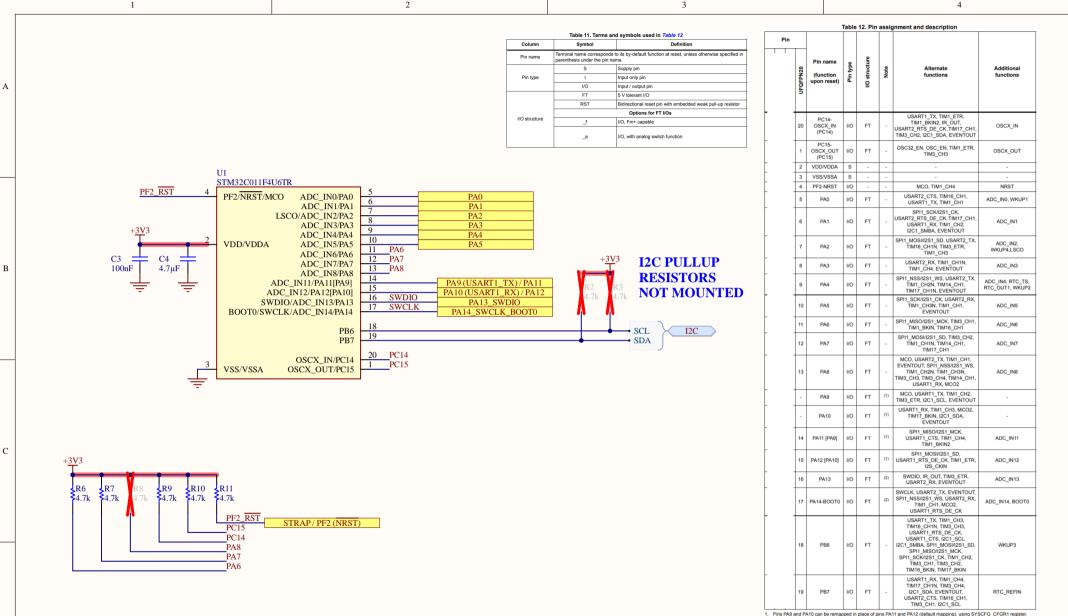
Upon reset, these pins are configured as SWD alternate functions, and the internal pull-up on PA13 pin and the internal pull-down on PA14 pin are activated. А
