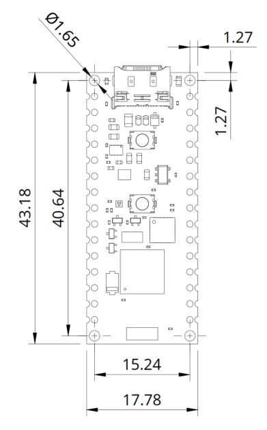
The Nano Matter has four 1.65 mm drilled mounting holes for mechanical fixing.
